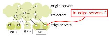
$\begin{array}{c} \text{adaptive streaming} \rightarrow \text{last-mile} \\ \text{edge servers in ISP} \rightarrow \text{peering link} \\ \text{commoditized hardware} \rightarrow \text{server under-provisioning} \end{array}$
